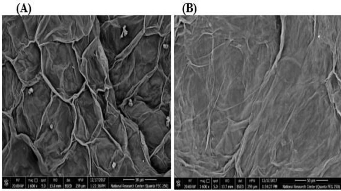
Figure 2: Scanning electron micrographs of banana fibers. (A) Control before treatment with enzyme, (B) after one hour of treatment with polygalacturonase from *Streptomyces* sp. GHB5.
